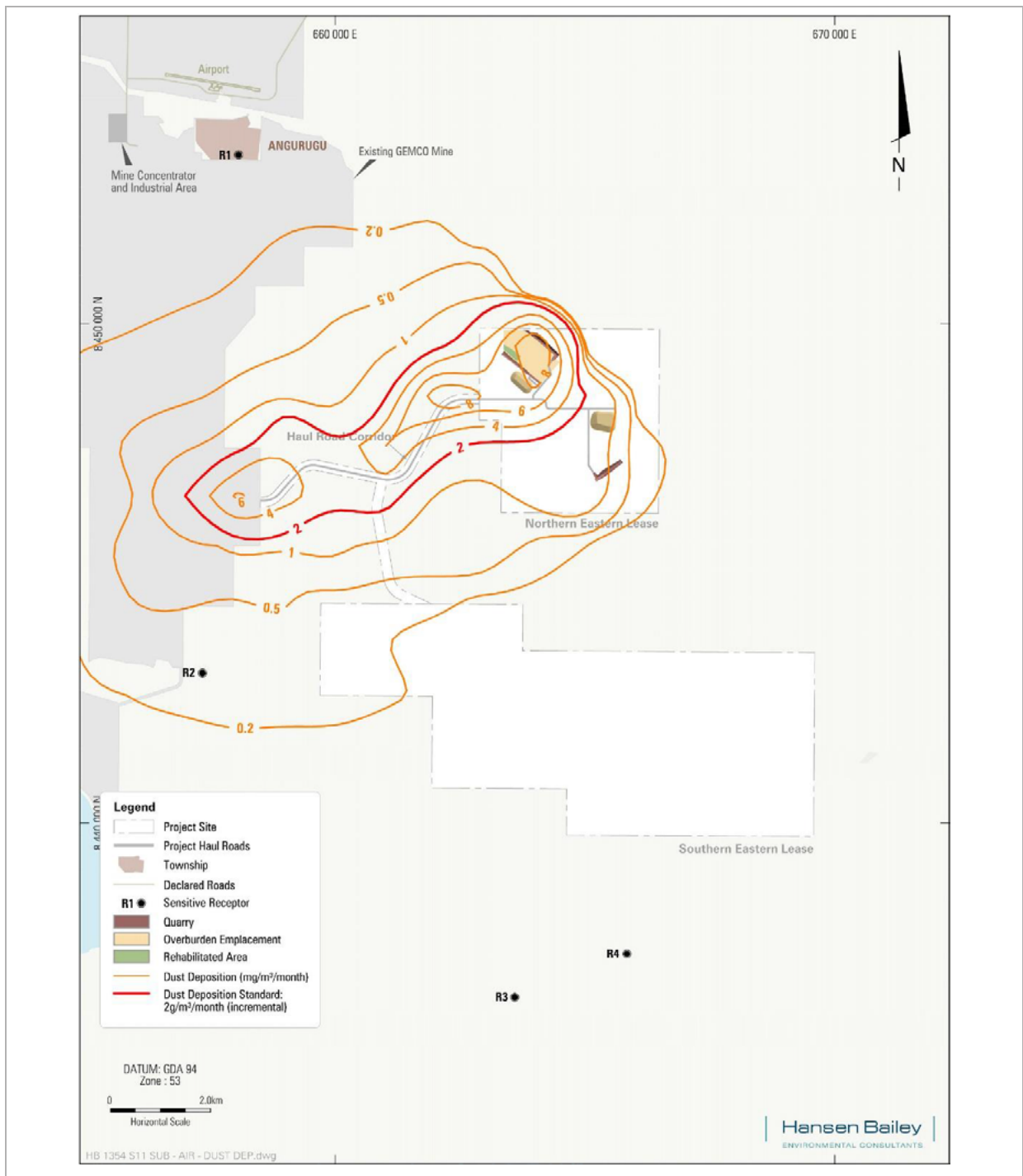
Figure 17 Project Year 3 Predicted annual average dust deposition rate due to the project in isolation
