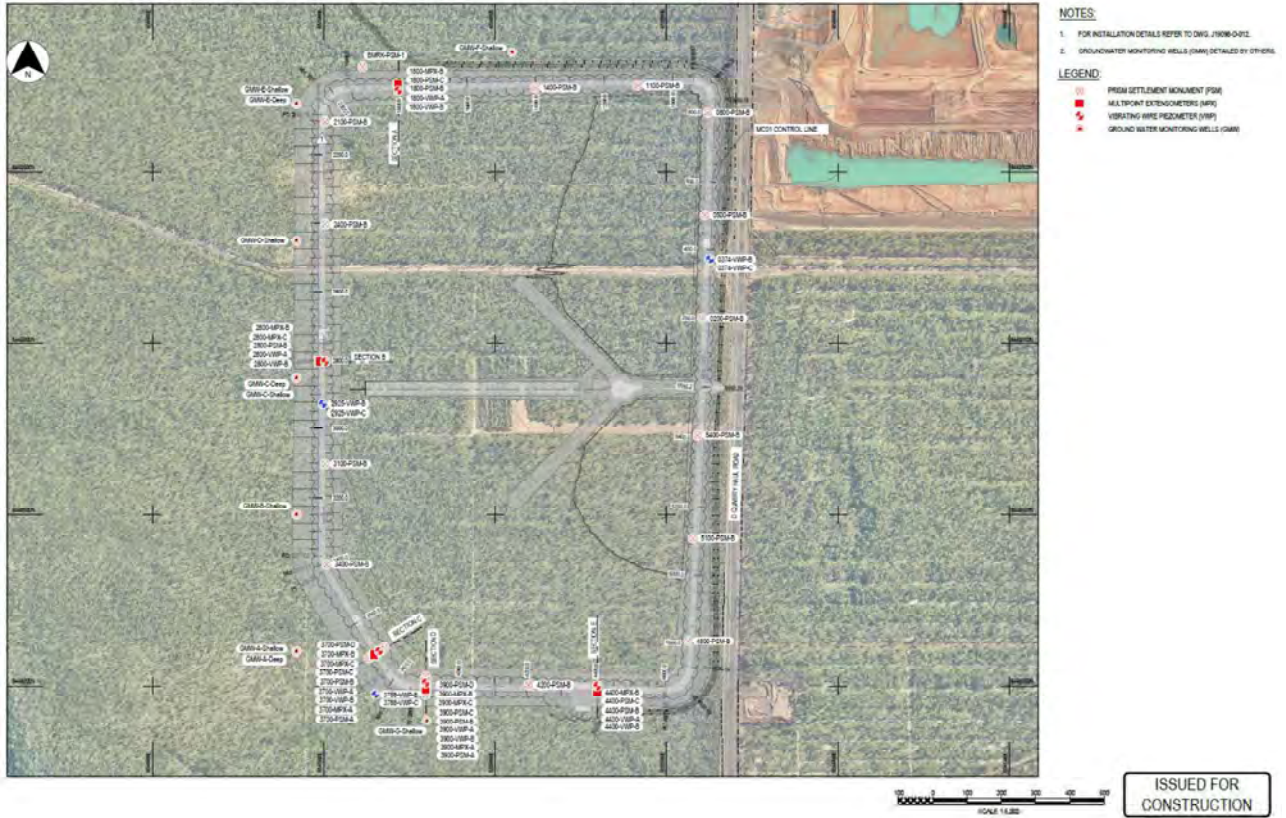
Figure 8 – Instrumentation and Monitoring Locations
